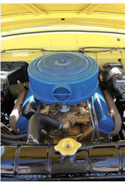
New to the 1956 model year was Ford's venerable 312-cu.in. V-8 engine, which helped Mercury set 20 performance records on Daytona's beach. Coupled with a Merc-O-Matic, it made 225 hp.
