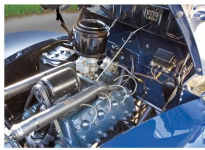
The De Luxe model's new "helmet" hood offered simpler access to the legendary flathead Ford V-8 engine.
