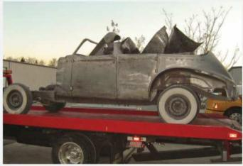
After moving the partially disassembled car down South, one of the first tasks was to have the body media blasted, work which was done while the body was still on the chassis, save for the bolt-on pieces. This revealed previous brazing.
