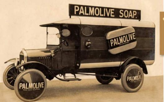
This van featured a fancy roof sign and three-dimensional panel for the body side, along with metal discs fitted over the wood-spoke wheels. All lettering of the well-known soap company's name was done by hand. This was one of the few trucks that also had a plated radiator shell and headlamp rims.
