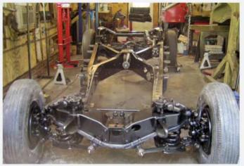
The chassis was completed in three months following its separation from the body. Shown here with the suspension, brakes, wheels, tires, driveshaft, and rear end installed, the chassis also displays Buick's then-innovative four-wheel coil-spring setup.
