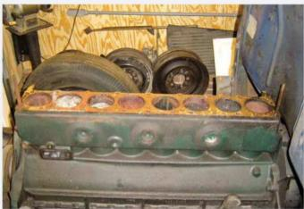
Along with the body and chassis needing complete restoration, the engine also required a complete rebuild. Though suffering from corrosion and other maladies, the engine was still suitable for machining and rebuilding.
