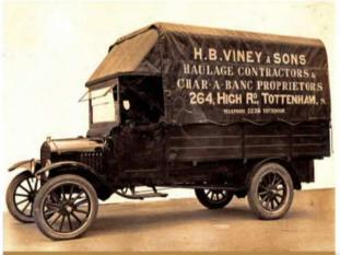
For this moving company, a Model TT truck was built using a wood bed with a removable canvas top. Note how the canvas top over the driver's compartment was separate from the bed section.
