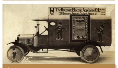
The Hotpoint Electric Appliance Co. Ld. panel van was painted in bright colors with the company's cartoon characters on the side. Note the metal wheel covers fitted over the wood-spoke wheels.
