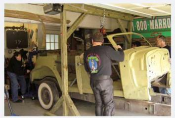
For the process of removing the body from the chassis, friends were recruited and used both the gantry and an engine hoist to make a smoother effort of the chore, and were able to roll the chassis out underneath the suspended body.
