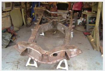
Separated from the body and with the suspension and braking components removed, the frame with Buick's strong "girder X-type" design (clearly visible here) was stripped to the bare metal for refinishing and reinstallation of the other chassis components.
