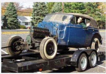
In the years before he moved the Buick to North Carolina in 2004, Brian and his father had partially disassembled the car, including removing any bolt-on body panels and much of the auxiliary engine components.
