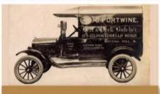
A Model T passenger car chassis was fitted with a panel body for the butcher to make deliveries. Note the fold-down windshield and oval window.
