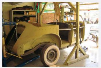
In order to hold the body once it was removed from the chassis, this gantry was made out of 6 x 6 lumber. Notice the body here has been covered in an etching primer to prevent any corrosion to the previously media-blasted surface.
