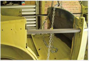
Despite the chains holding the body to the gantry (and eventually saw horses below supporting it), the convertible body, minus its doors, needed additional structural strength. So, four angle-iron supports were welded in between the door pillars.
